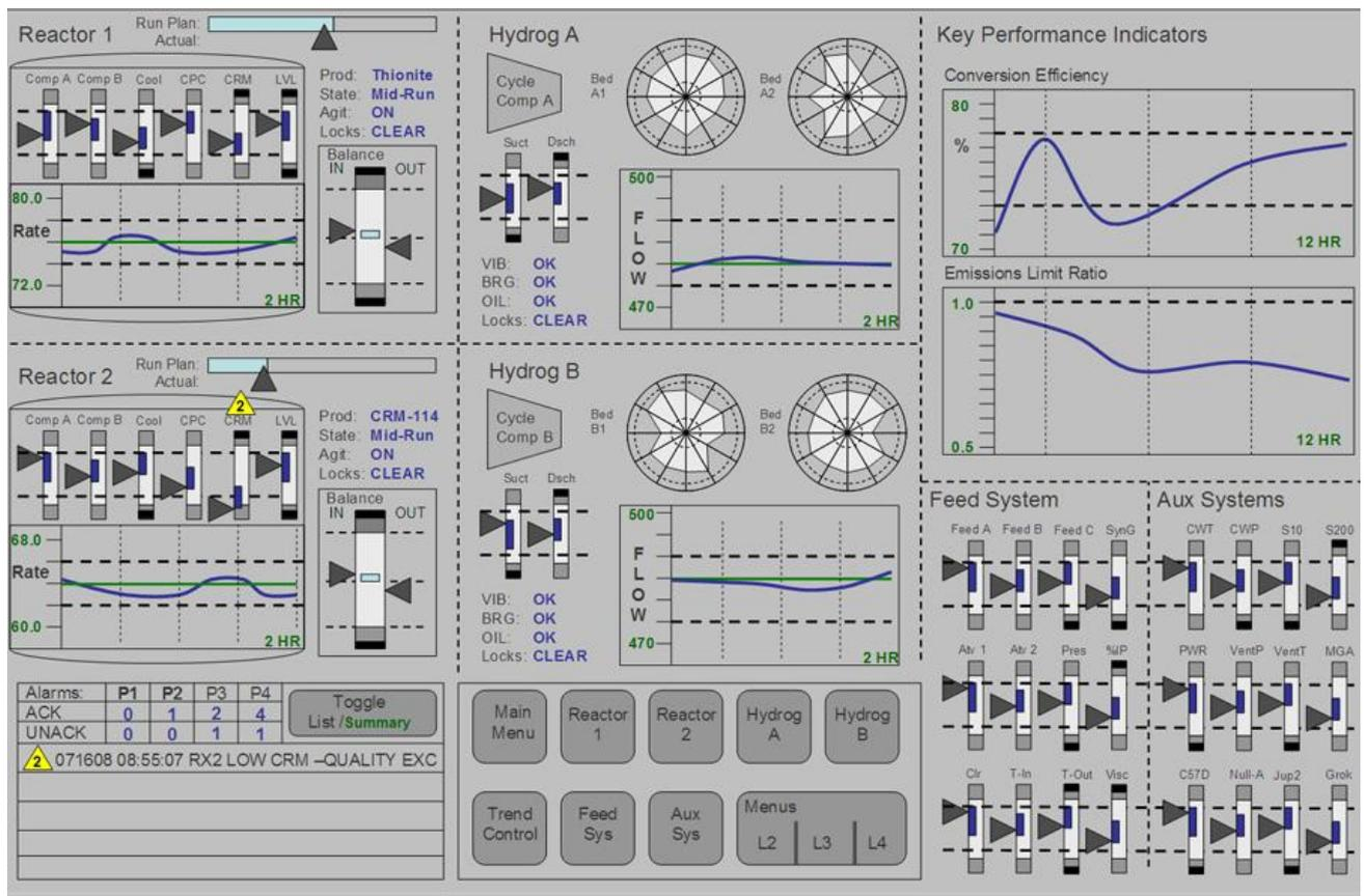
Figure 3.3 HPHMI process overview display with graphic elements representing important key variables. From Hollifield et al. (2008), page 101.
