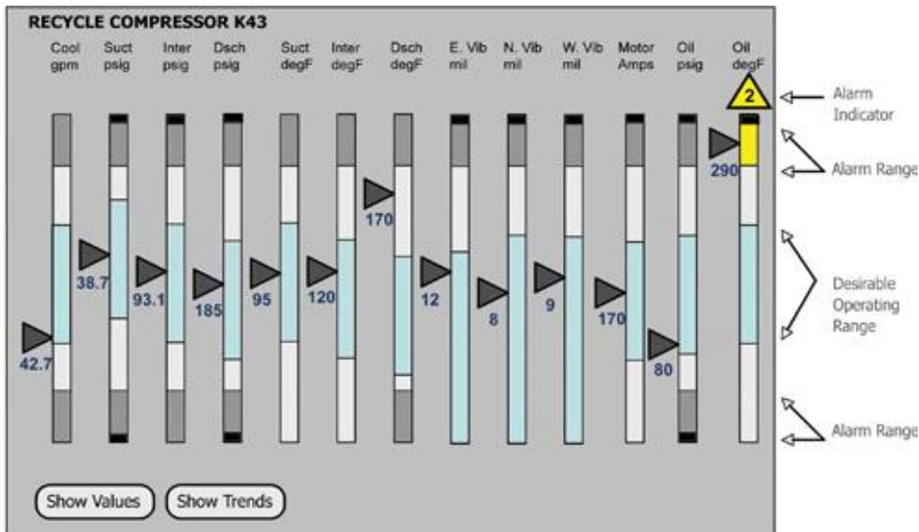
Figure 2.5 Presentation of process status with bars and moving analog indicators that shows the current level. From Hollifield et al. (2008), page 59.
