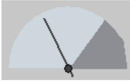
Figure 4.4 Visualization for values that must not exceed a certain limit. Alarms are presented according to the color scheme in the basic level indicator.
