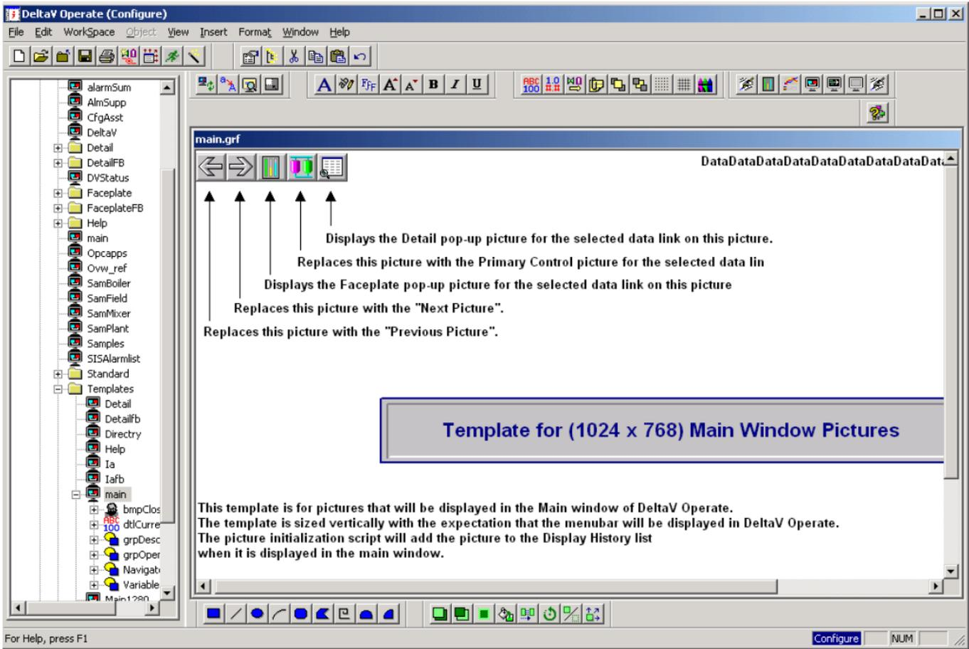
Figure 3.4 DeltaV Operate configure mode in Windows setting. System tree to the left and work area to the right. From the DeltaV manual "Getting Started With Your DeltaV Digital Automation System". Emerson Process Management (March, 2006).
