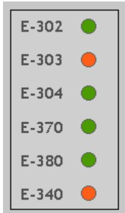
Figure 4.7 Table-like visualization of centrifuges operating mode. Green = automatic mode, orange = manual mode.
