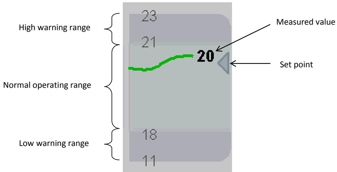
Figure 2.3 IRD building block of a separator. From Braseth et al. (2004), page 9.
