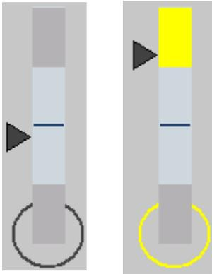
Figure 4.3 To the left: Temperature indicator without alarms active. To the right: First warning limit is surpassed. If there exists a critical limit it is presented in red.
