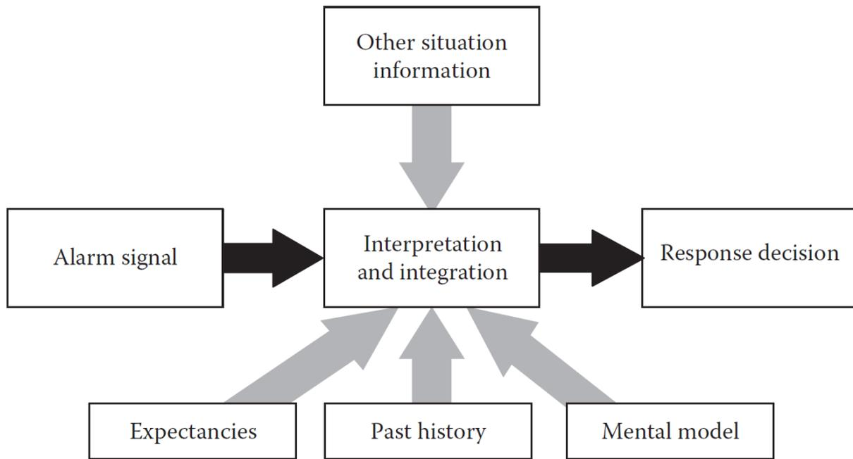
Figure 2.2 Mental process when responding to an alarm. Many things are taken into consideration. From Endsley & Jones (2011), page 149.
