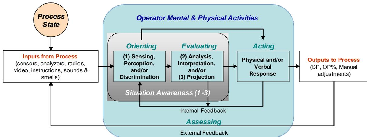
Figure 3.1 The mental process when gathering information about process state and then translating it into action and output to the process. From *Abnormal Situation Management (ASM) Visual Thesaurus Webinar “Using Qualitative Display Shapes for Improving Operator Situation Awareness”* (December 10, 2010), page 10. SP = set point. OP = output.
