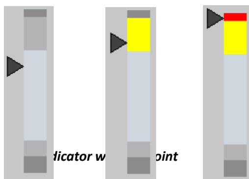
Figure 4.1 To the left: Basic level indicator without alarm active. Middle: First warning limit is surpassed. To the right: The critical limit is surpassed.
