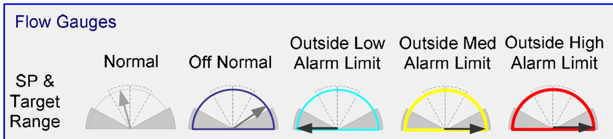
Figure 3.2 Appropriate visualization of a flow gauge in its different states. Arrow depicts the current value. Dotted lines shows target value range. From Bullemer & Reisin (2008), page 12.
