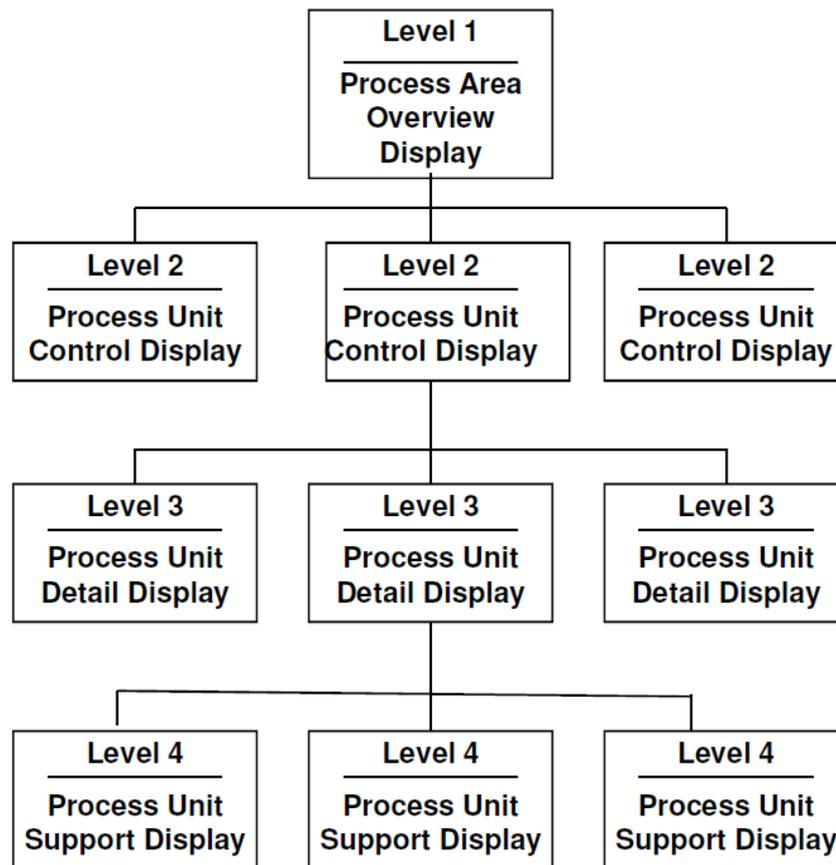
Figure 2.1 Schematic overview of the interface hierarchy. From Rockwell Automation presentation “The High Performance HMI”.
